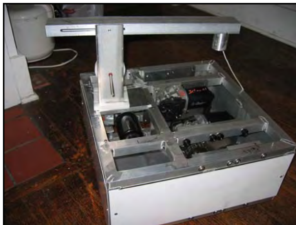
Figure 2 Topless Zippy without electronics
